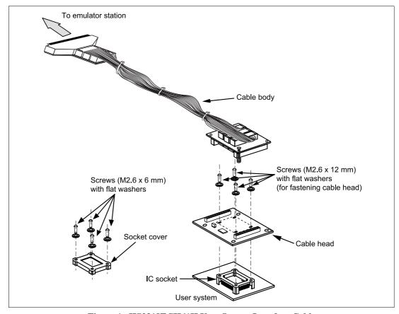
Figure 1 HS2318ECH61H User System Interface Cable
